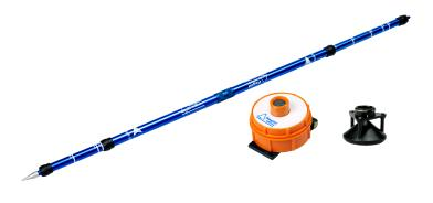
The Transponder T3 has a water resistant and rugged construction in a bright, visible color. T3 uses one AA battery and it is compatible with Haglöf instruments DP DME, Vertex IV, DME and Vertex Laser. The transponder is equipped with a sharp pin and can be placed directly on a tree stem. It can also be used with an adapter and monopod staff to measure in a full circle in sample plot work.
