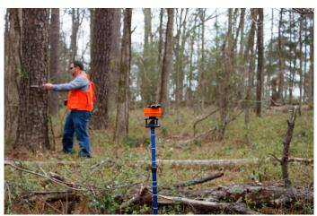
Position the T3 transponder in the plot centre on the monopod staff. The monopod, used for the DP DME, the Vertex IV, the Vertex Laser and the DME, is customized for use in tough field conditions. Measure the tree diameter with the caliper and activate the DP DME in your computer terminal. The software will determine the distance from the tree centre to the plot centre.
