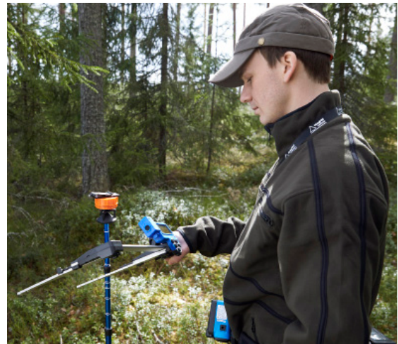
Haglöf Sweden's DP II caliper works with different software-run add-ons and accessories, designed to improve accuracy, efficiency and versatility. With add-on instruments mounted on the DP caliper com-port, battery and display are supplied from the caliper.
